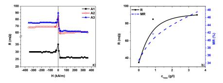
Figure 5.1: R = f(H) curve (a) and (b)  $R = f(c_{TiO2})$  and  $MR = f(c_{TiO2})$  curves for A1, A2 and A3 films [1]
