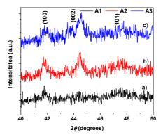
Figure 3.1: XRD patterns (enlargement for the region of Co lines) for the films: a) A1, b) A2 şi c) A3 [1]
