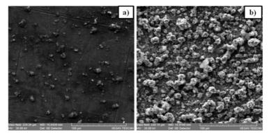
Figure 3.2: SEM micrographs for the films: a) H1 (1.1 A·dm<sup>-2</sup>) and b) H2 (3.2 A·dm<sup>-2</sup>) [4]
