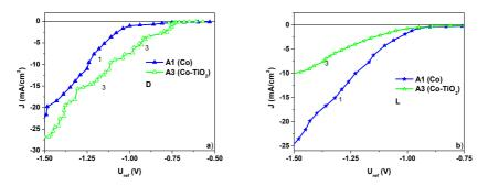
Figure 5.4: The J = f (*Uref*) curves drawn in the dark (a) and under UV radiation (b) for A1 and A3 samples
