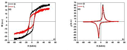
Figure 5.3: M = f(H) (a) and  $\chi = f(H)$  (b) curves for H3 sample
