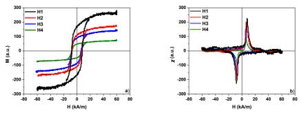
Figure 4.1: The curves M = f(H) (a) and  $\chi = f(H)$  (b) for H1, H2, H3 and H4 samples [4]
